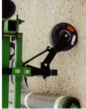
Our spring-loaded fabric guide wheels are adjustable to ensure proper seating of the fabric edge in the trench.
